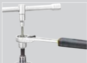
Fitting shock absorbers usually requires a 22mm socket.
