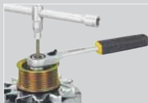
The pulley on an alternator will usually have a 24mm nut.
