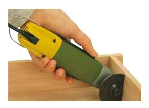
For precision square excavations, HSS immersion saw blades are available with an 8 and 14mm width of cut.
